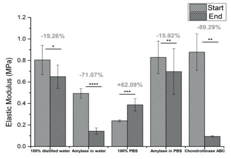
Fig. 2. Results of mechanical properties measured with AFM Peakforce QNM.
